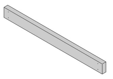
Optional: pre dril 1/8" holes for screws to mount ladder rungs to posts appoximately as shown both ends
